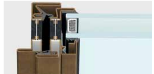
lateral section | frame section 47 mm
