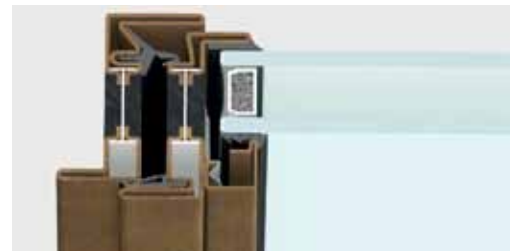
lateral section | frame section 47 mm
