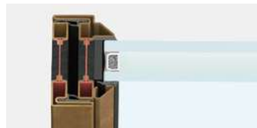
lateral section | frame section 47 mm
