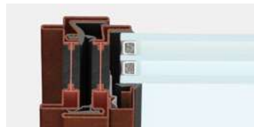
upper side section | 62 mm visible section
