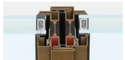
central section | frame section 62 mm
