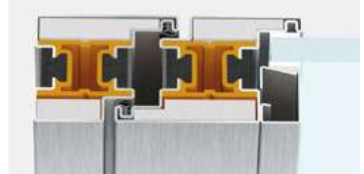
lateral section | frame section 134mm
