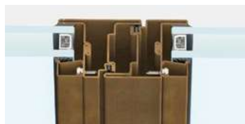
central section | flush | frame section 101 mm
