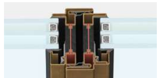
central section | frame section 62 mm
