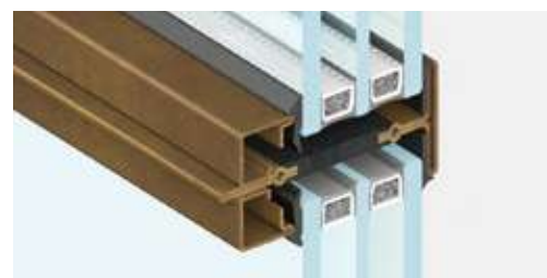
glazing bar | frame section 36 mm
