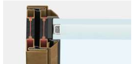
lateral section | frame section 47 mm
