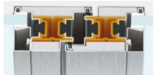
central section | frame section 156 mm
