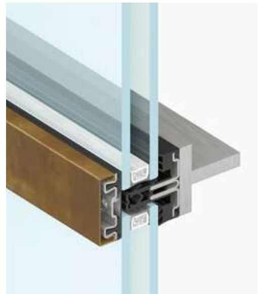
application to transom | 50 mm face section
