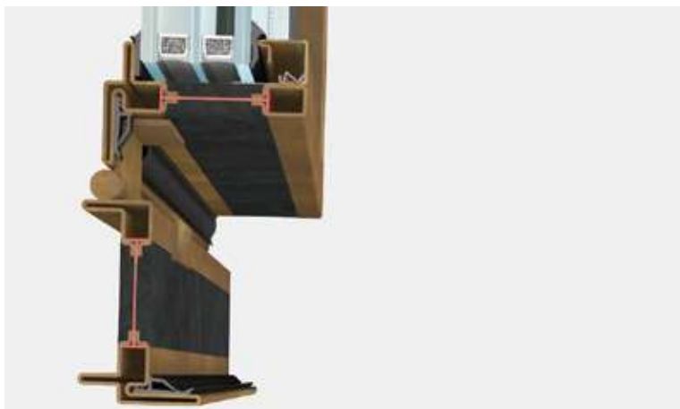
lateral section | frame section 47 mm
