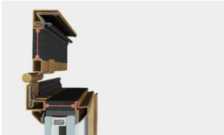
lateral section | frame section 47 mm
