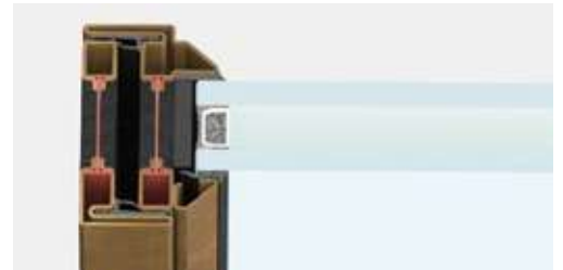
lateral section | frame section 47 mm
