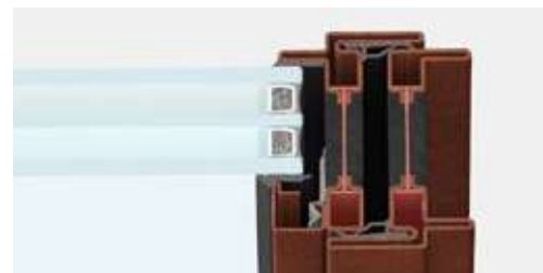
upper side section | 62 mm visible section
