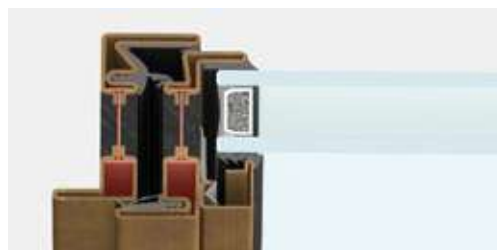
lateral section | frame section 47 mm
